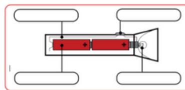
The lamps show below do not work. Circle the cause of the failure in each case.
